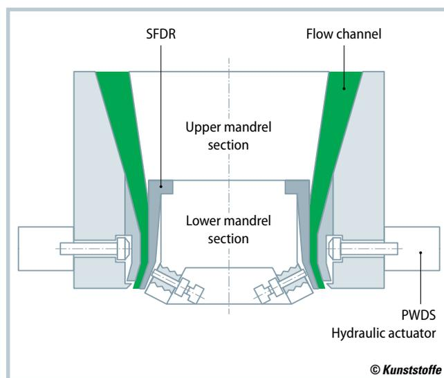
**Fig. 1.** Partial wall thickness control (PWDS): Actuators guide a static flexible deformable ring (SFDR) to change the die gap (source: [2])
