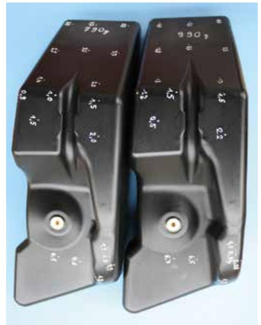
**Fig. 6.** Weight and thickness distributions of a windshield washer reservoir produced with a GWDS wall thickness control die (left) and conventionally (right) (© H. Gross)
