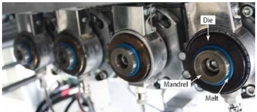
**Fig. 4.** GWDS wall thickness control dies with a diameter of 40 mm integrated into a fourfold head. The cylindrical mandrels shaped at the end have been extended from the die here since the shaping is not needed for this section of the component (© H. Gross)
