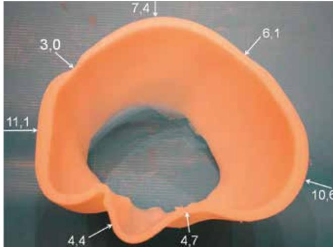
**Fig. 3.** Unstretched, cooled parison from a GWDS wall thickness control die: Notwithstanding the different wall thicknesses (in mm), the parison came out of the die sufficiently straight to hit the blowing mandrel (© H. Gross)
