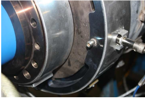
Fig.2 Tulting die in operation showing one of the small axially arranged adjusting screws having a special fine pitch for a sensitive tilting of the die
