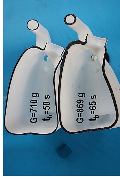
Fig. 4 Part produced conventionally (bottom), Part produced with GWDS (top)
