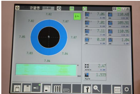
Figure 6 Photo showing the excellent centricity that has reached with the help of the tilting technology
