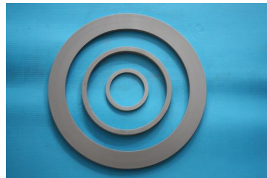
Figure 1 Rubber tilt joints of different geometries which seal the dividing plane between the die and the head and which in the same time allow for a sensitive tilting of the die
