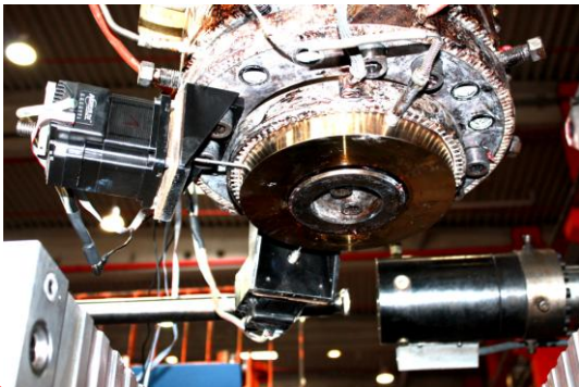
Figure 3 Head for extrusion blow molding retrofitted with a tilting die which is adjusted by two stepper drives arranged in a 90 degree angle to reach every relative position in regard to the pin
