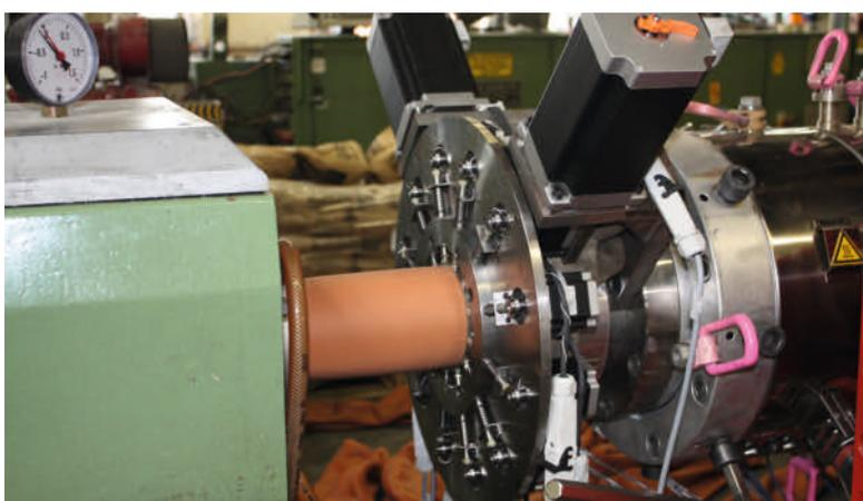
**Fig. 5. Flexring tool used for the tilting technique – for the first time, it is thus possible to conduct closed-loop control of eccentric, as well as asymmetric variations in thicknesses**
