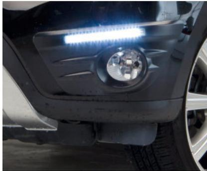
Daytime running lamp covers made out of matt, scratch resistant PMMA (photo: Mitras)
