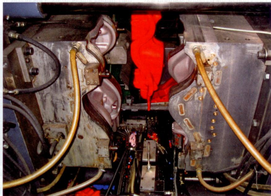
Fig. 1. The Bobby Car being removed from the mold at the end of cooling (photo: BIG)
