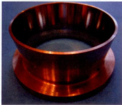
**Fig. 2. One-piece Flexring sleeve with a diameter of 130 mm in which the 15 individual walls of the flexibly deformable conical region mutually support one another**
