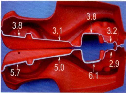
Fig. 5. Comparison of wall thickness distributions (in mm) in the bottom region of the blow molded item produced using the Flexring die (above) and using a conventional die (below)
