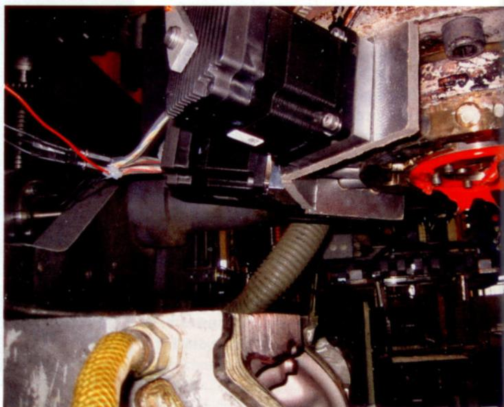
**Fig. 4. Flexring die installed on the production equipment during the optimization trials (photo: BIG)**
