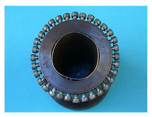
Fig. 1 Cross sectional drawing of a flexring Die (right side) and Photo of an outer ring with an integrated flexring sleeve (left side)
