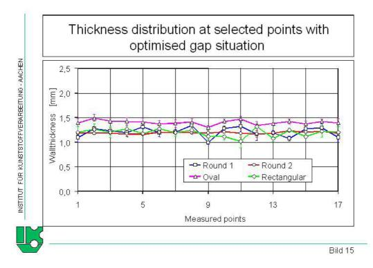
Fig. 7 Wall-thickness distribution in the sectional planes with optimized static sleeve deformation (source IKV [2])
