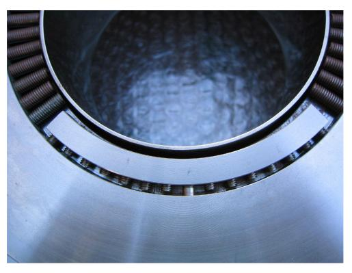
Fig. 3 Adjustment jaw with integrated grub screws for fine setting of the active setting jaw contour
