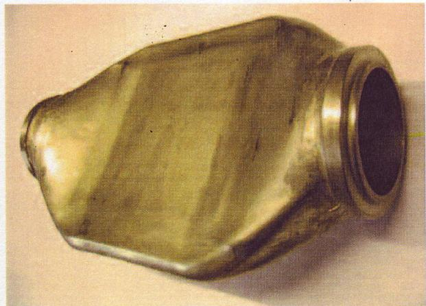
Fig. 7. Throttle body with the continuous transitions from the central flat flow-channel geometry to the respective circular inlet and outlet geometries
